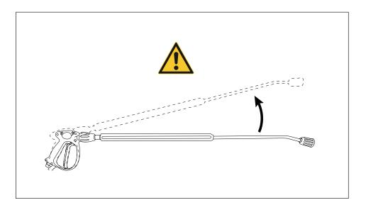
Fig. 6 - 2 Recoil force when switching on the trigger gun
